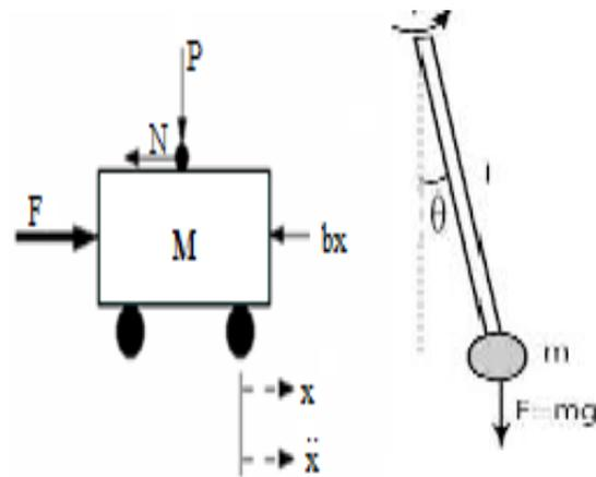
Fig. 1 Inverted Pendulum System and Free body diagram
