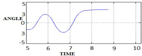
Fig 2 Swing up of inverted pendulum
