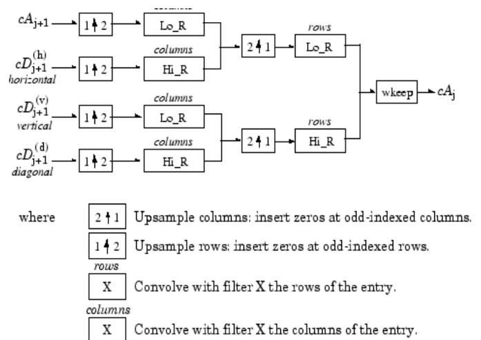
Fig3. 2-D Inverse Discrete Wavelet transforms
