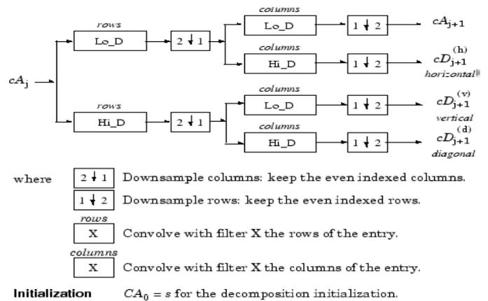
Fig2. 2-D Discrete Wavelet transforms
